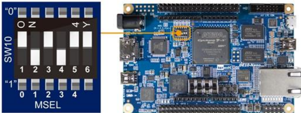
Figure 7-3 Set MSEL[4:0] to "01010" for ARM Version Mode
