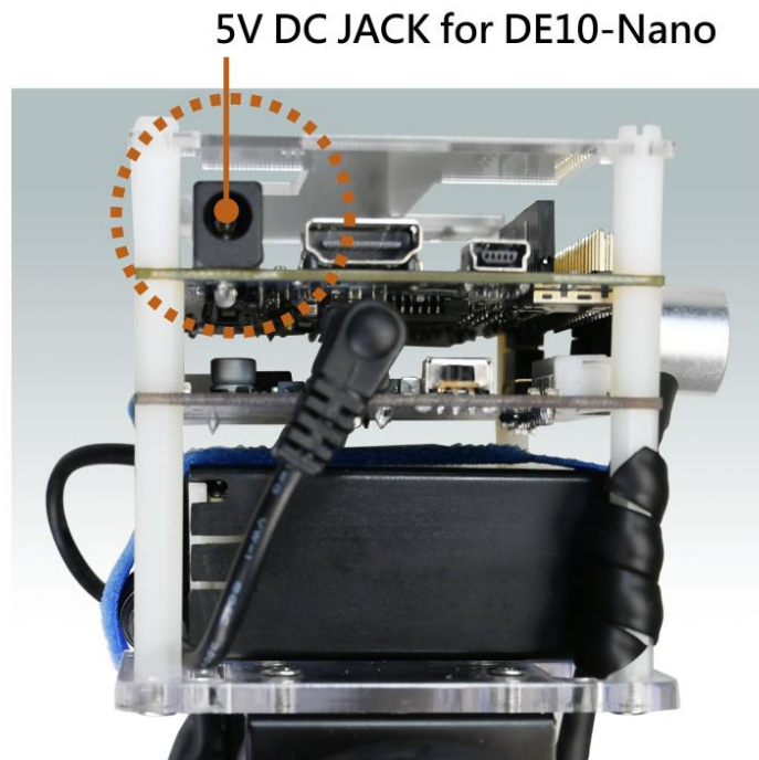
Figure 3-14 5V DC power jack for DE10-Nano board
