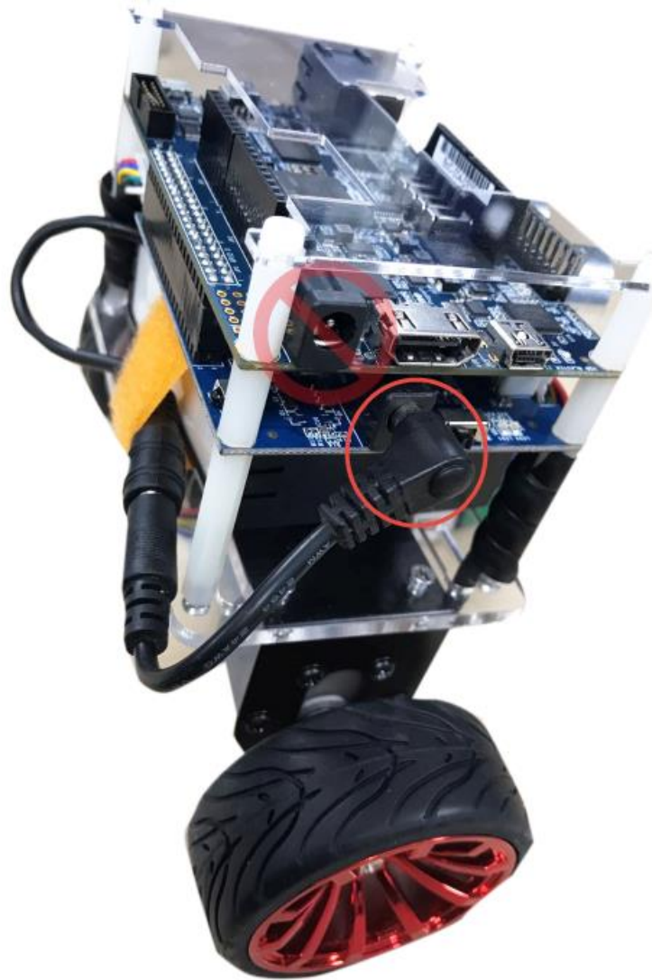
Figure 3-15 Connect DE10-Nano Power JACK to 12V Battery is banned
